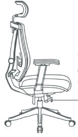
Rotate this handle clockwise to increase back tilt tension.
