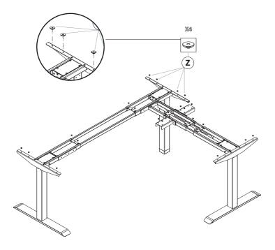
9. With a partner, carefully place Desktop (D) into position on top of the frame. Then, fix Desktop (D) into place using  $28 \times (Y)$  Screws in the positions indicated. Unscrew 4 Screws on the frame. Place  $1 \times (X2)$  Spring Washer and  $1 \times (X1)$  Plain Washer on each (M1)Screw, then use them to fix the
