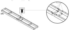
4. Extend Support Beam (H) and place over the remaining Side Leg (A). Fix into place using 4 x (W) Screws.
