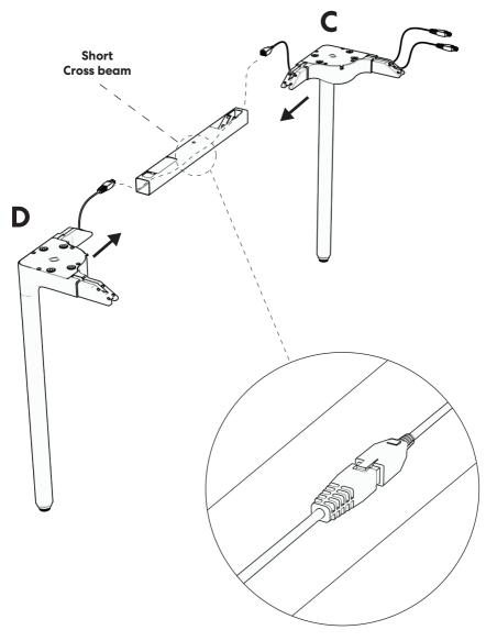
**Note:** After connection, put the cable and the cable head into the **Short Crossbeam.**
