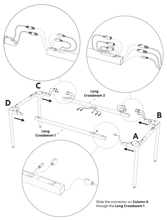
Note: After connection, put the cable and the cable head into the Long Crossbeam 2.
