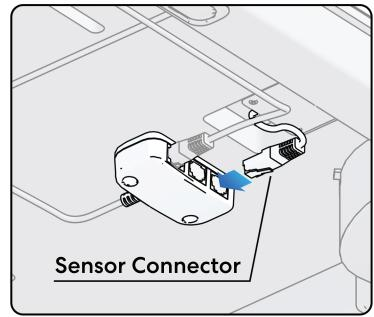
2. Use a screwdriver to attach the **Splitter** to the **surface** with 2 **screws (D)**, then connect the **Sensor Connector** to the **Splitter**
