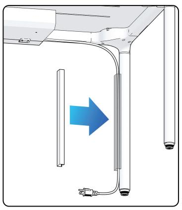
1. Put the Main Power Cord into the Upper Tube, attach the Upper Tube to the Column B
