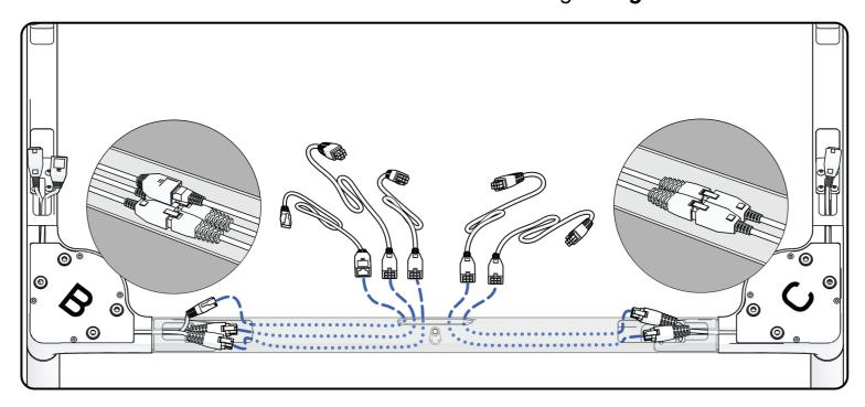
**Note:** After connecting, place the **cable** and **cable head** into the **Crossbeam**
