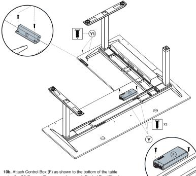
using 2 x (Y) Screws. Or you can place each Control Box (F) onto the corresponding Cable Tray (L).
