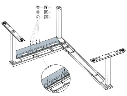
$\pmb{8a.}$  Flip the frame upright. Attach 3 x Brackets (E) to the end of the Support Beams using 2 x (W) Screws for each Bracket.
