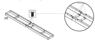
4. Extend Support Beam (H) and place over the remaining Side Leg (A). Fix into place using 4 x (W) Screws.
