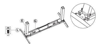
4. Fasten the foot (H) and legs (A) with M6x14mm (L) screws.
