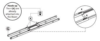
2. Attach Legs (A) to the Support Beams (G) using 8 (K).
