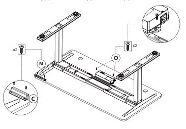
7. Fasten the control switch (C) and desk top (D) with ST4x20mm (M) screws.
