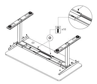
6. Fasten the desk top (D) and the control box (B) with ST5x20mm (O) screws.
